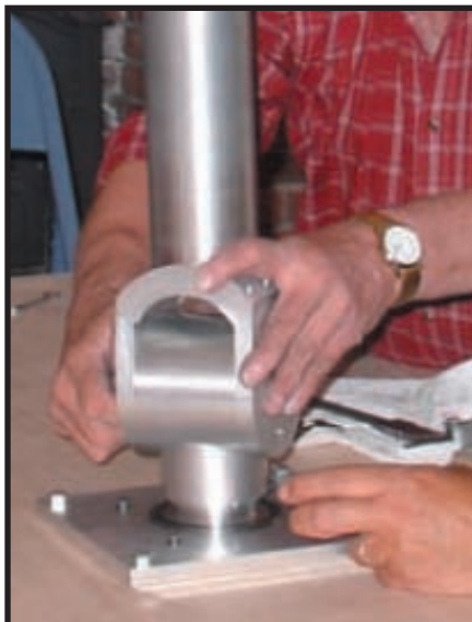
Photo 3 —The Vision-Arm's shoulder (Smart Robotics) consists of rotation and pivot joints. Machined aluminum parts keep weight down to a minimum.
