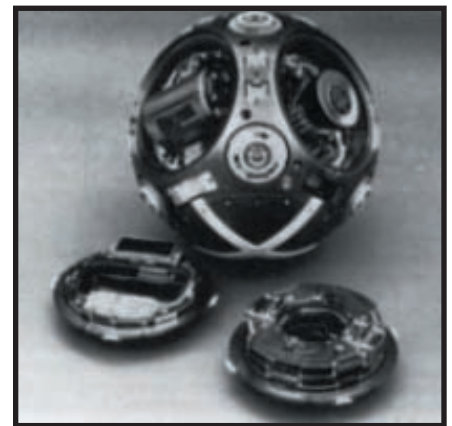
Photo 1 —The golden age of mechanical inertial navigation systems is represented by the Advanced Inertial Reference Sphere. That's "golden age" as in "price is no object." It's reported that AIRS contained 19,000 parts and each accelerometer alone cost $300,000 and required six months to manufacture. [2]
