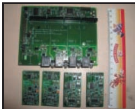
Photo 1 —Here you see the 4fx daughter board and modules before assembly. Each of the four modules at the bottom mate with matching connectors in the middle of the 4fx daughter board. Note the large vacant area in the middle of the PCB. It is necessary to provide physical isolation between the FXO ports and the rest of the system.
