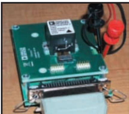
Photo 2 —This is an Analog Devices ADIS16350 evaluation board. In 1953, there was much ado about the "Navigator in a closet" designed by scientists at MIT. Today, thanks to MEMS accelerometers and gyros, the '16350 offers the prospect of a "Navigator in a matchbox."
