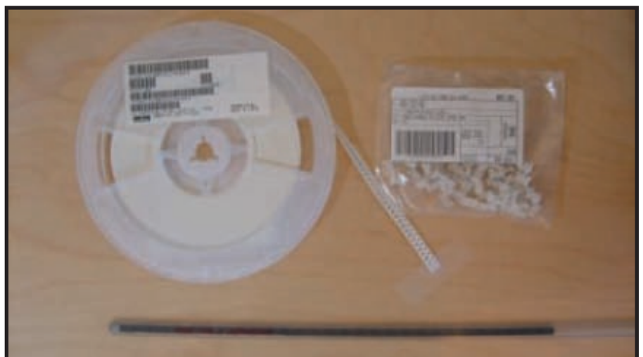
Photo 4 —Here is a reel of tape with resistors, a tube containing microchips, and a bag of bulk connectors. The tube and reel are standard sizes and can be fed into most assembly machines. The bulk connectors will have to be placed by hand.
